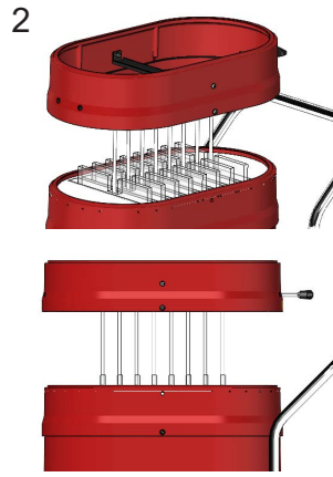
2 Place in the filter cage housing spacer assembly, making sure to keep the ground wire flat.
