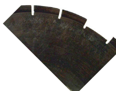
Segment Loss: Usually insufficient water
