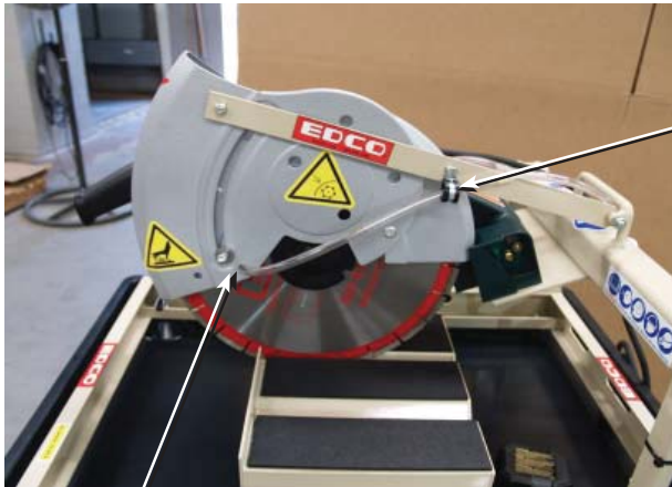
Insert end of 14" hose in this hole
