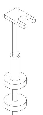
BIT REMOVING TOOL (SLIDE HAMMER) PART # 63220
