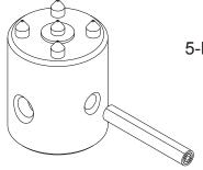
5-POINT TUNGSTEN CARBIDE BIT WITH COILED SPRING PIN PART # 18810 5 REQUIRED
