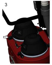
Loosen the motor retaining knobs enough to remove motor under negative pressure.
