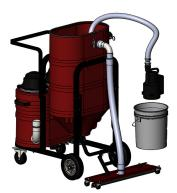
Place the pump in a 5 gallon bucket and run the clean water through the pump.
