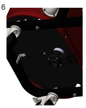
Open the slidegate under the filters to empty any liquid from the filter chamber. Close the slide gate before using the unit.
