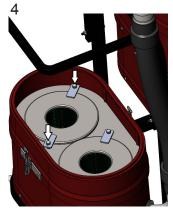
Loosen filter hold down bracket bolts enough to remove the filter.
