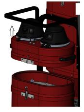
Remove motordeck and inspect filter. The filter is used to stop moisture from entering the motor and not for filtering dust.
