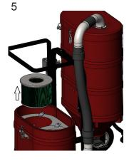
Remove filter and inspect. Replace filter as needed to maintain optimal performance.
