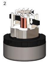
Remove motor fan cover by pressing down on clips located on each side.
