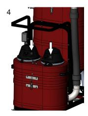
Turn machine off using the ON / OFF switch on the motor domes.
