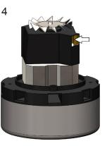
Carefully dislodge the plastic motor cap via the built-in hooks on both sides of motor brush. (TIP: Dislodge one side of a cap first followed by the other.) With a flathead screwdriver, flip brush tab upward. Use pliers to then pull the brush out by the tab.
