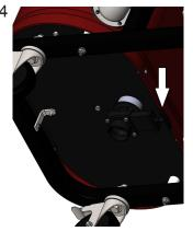
Use the internal pump to evacuate the water. You must hold the switch down to operate the pump.
